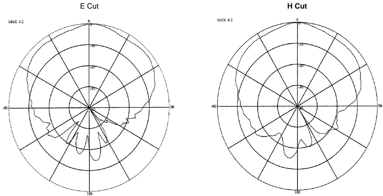
Figure 2-2. Far Field Plots Azimuth Cuts
